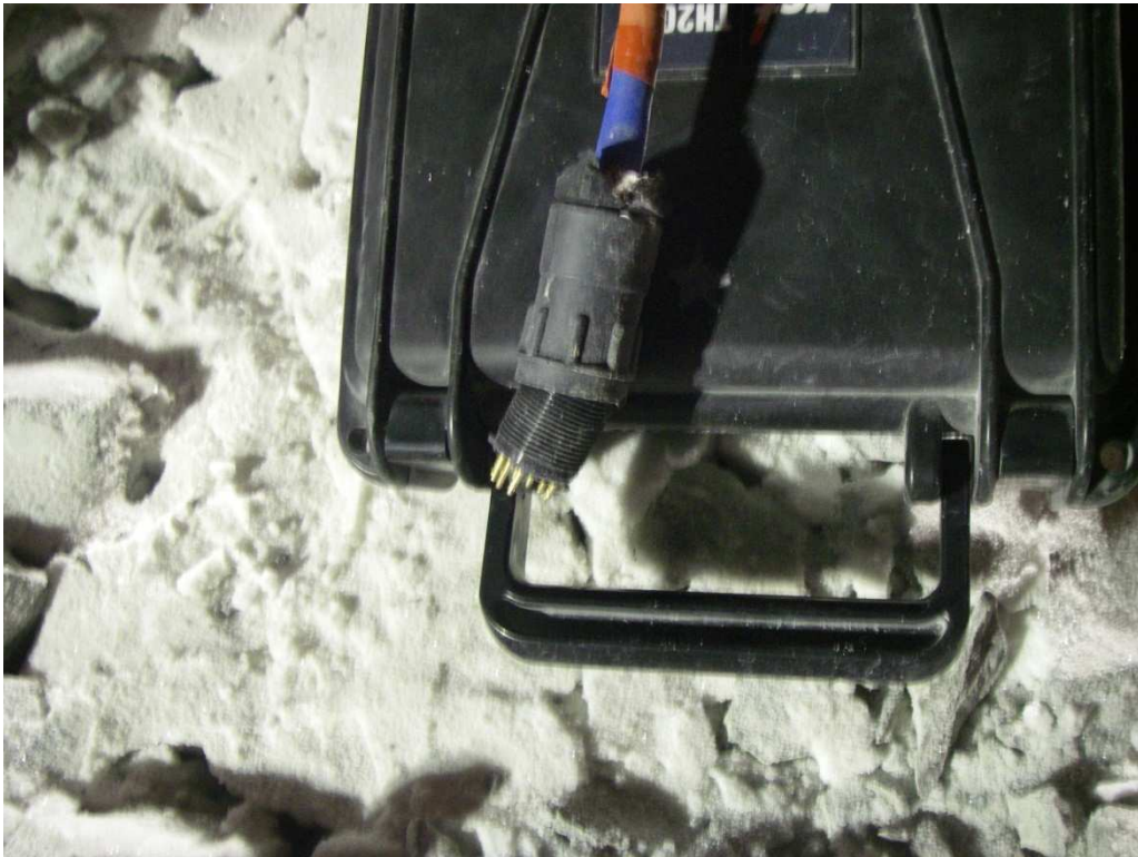
Photo 11: Broken thermistor connector.
