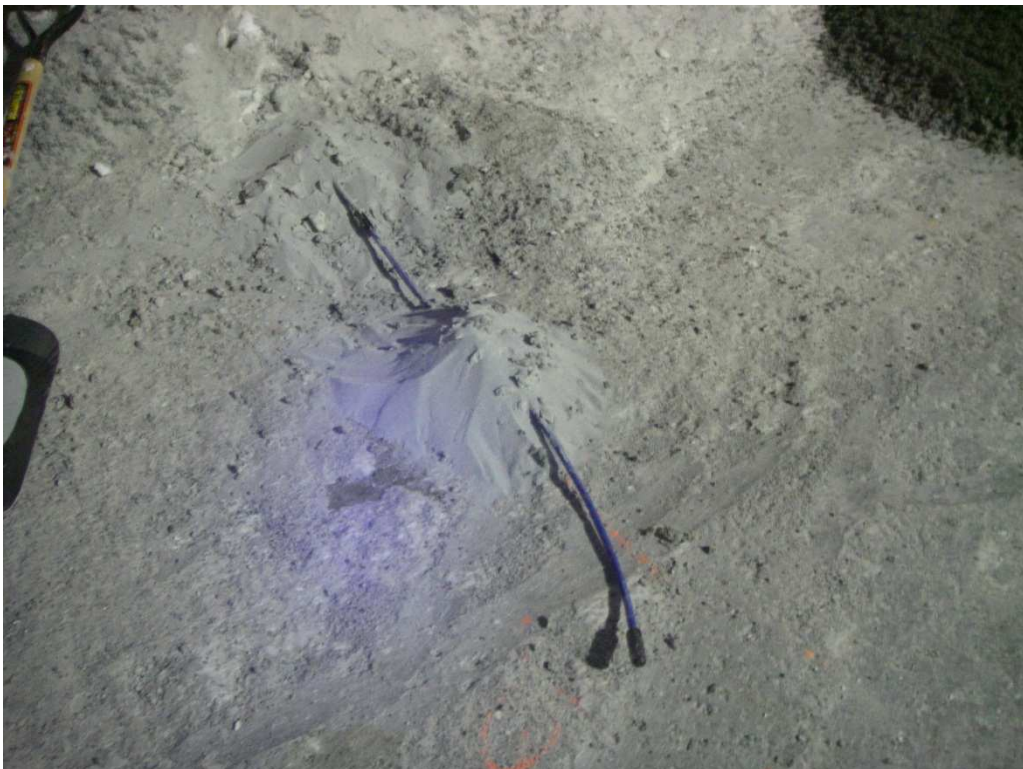
Photo 12: Last 2 beads of ND-HTS-175-33.5 before being buried in frozen core material.
